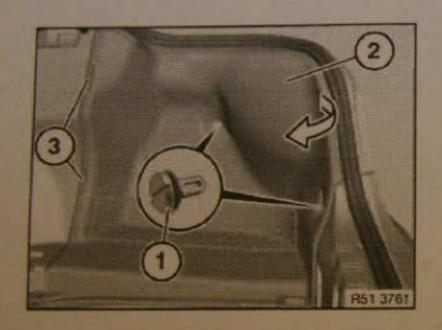
Open rotary clips (1) and remove.
