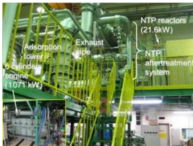
Fig. 2 Full-scale prototype for plasma aftertreatment system for marine diesel engines
